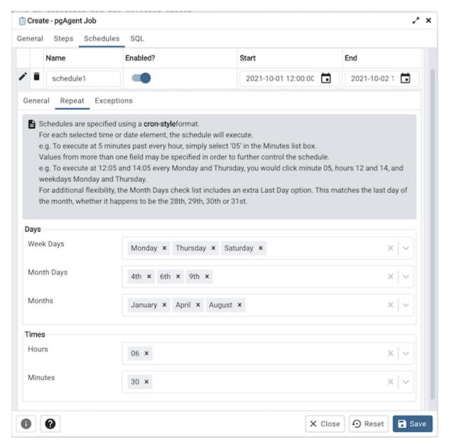
Use the fields on the *Repeat* tab to specify the details about the schedule in a cron-style format. The job will execute on each date or time element selected on the *Repeat* tab.
